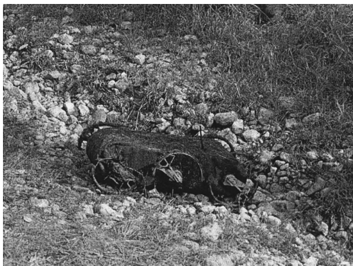
Figure 1.11: RHEX, a six-legged robot (Courtesy of G. Dudek, McGill University)
